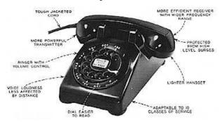
electrical components inside the set and should not be confused with "network" in "telephone network" which refers to the global interconnected system). If it is a two-piece set, the transmitter and receiver are mounted in the handset, the ringer is typically in the base, and the dial and
